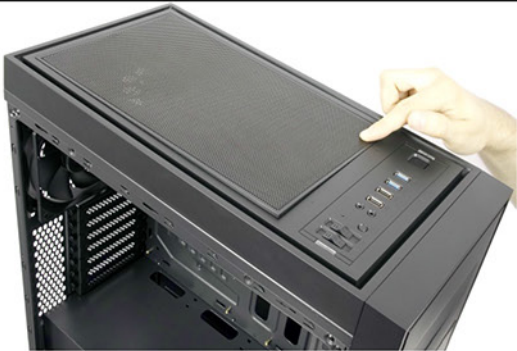
Push the top fan cover in the designated spots to release the locking mechanism
