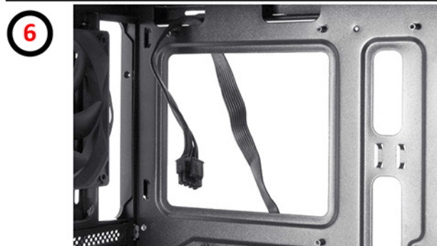
Lead the EPS cable through the dedicated hole
