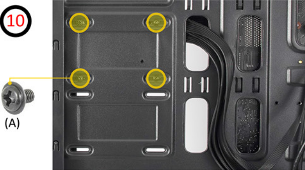
Secure the SSD in dedicated place using four screws (A)
