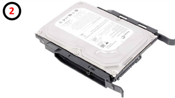
Insert the HDD into the dedicated mounting tray
