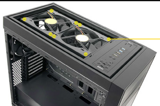
Install the 140 mm fans using dedicated screws (E)
