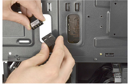
Plug the power connector from the fan controller to the 4-pin molex connector from the PSU
