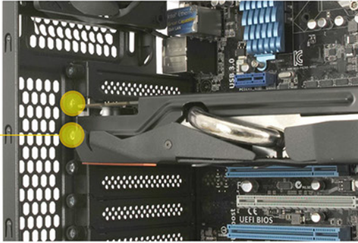
Install the GPU in the PCI-E slot on the motherboard and secure it with (F) or (B) screws
