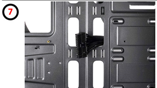
Lead the ATX cable through the dedicated hole
