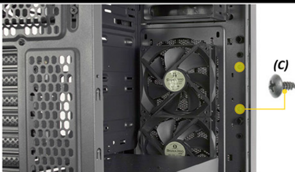
Secure the front panel using dedicated screws (C)
