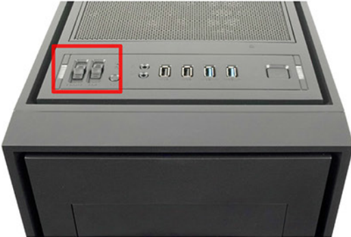
Two built-in fan speed switches
