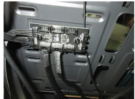
Place the fan controller within the computer case
