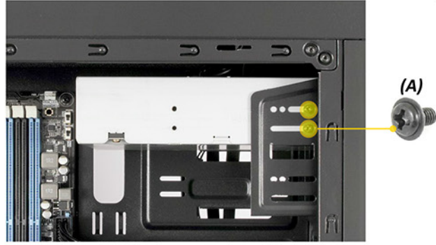
Remove the front 5.25" drive bay cover, then slide the ODD into the drive bay and secure it with screws (A)
