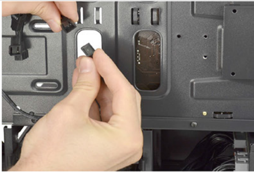
Plug in the 3-pin fan connector to the dedicated connector on the fan controller
