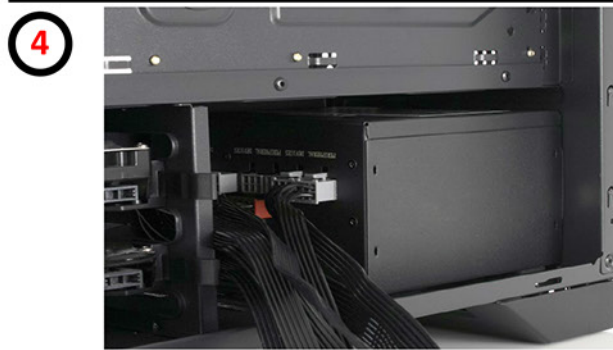
Position the PSU on the bottom of the case with the fan facing downwards
