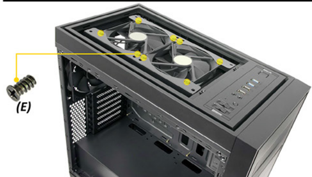
Install the 120 mm fans using dedicated screws (E)
