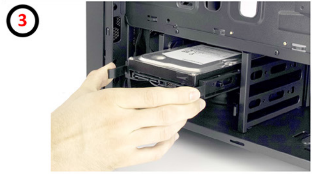
Slide the HDD into the HDD cage
